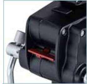
Safety lock for controlled raising and lowering
